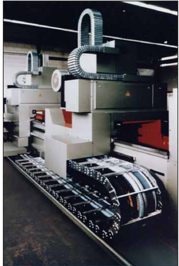
Product: VARITRAK S & CONDUFLEX Operating Mode: Horizontal (off & on-the-floor) and Vertical (loop-up) Application: Custom Machinery
