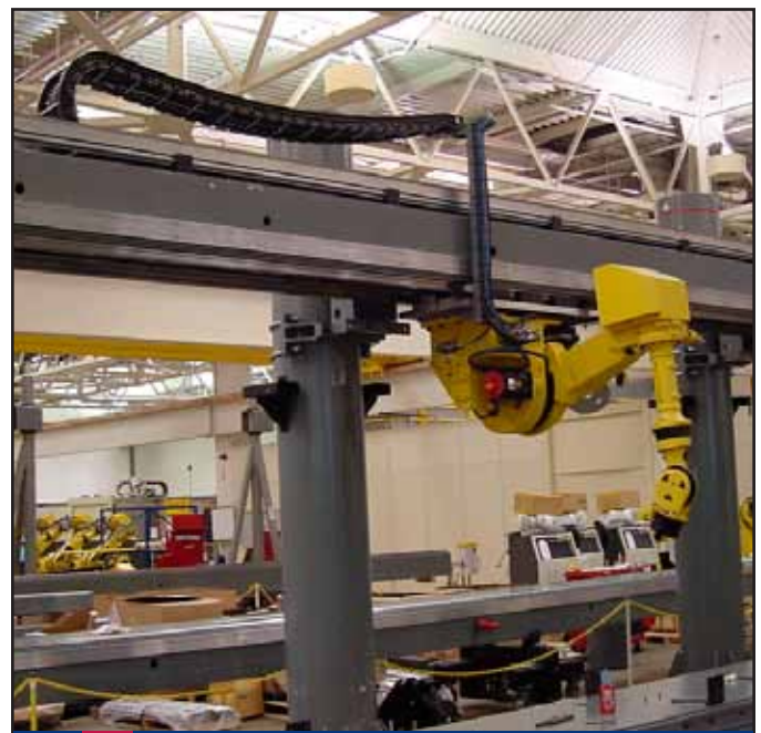
Product: QUANTUM Operating Mode: Horizontal (long-travel, off-the-floor) Application: Factory Pick & Place Automation
