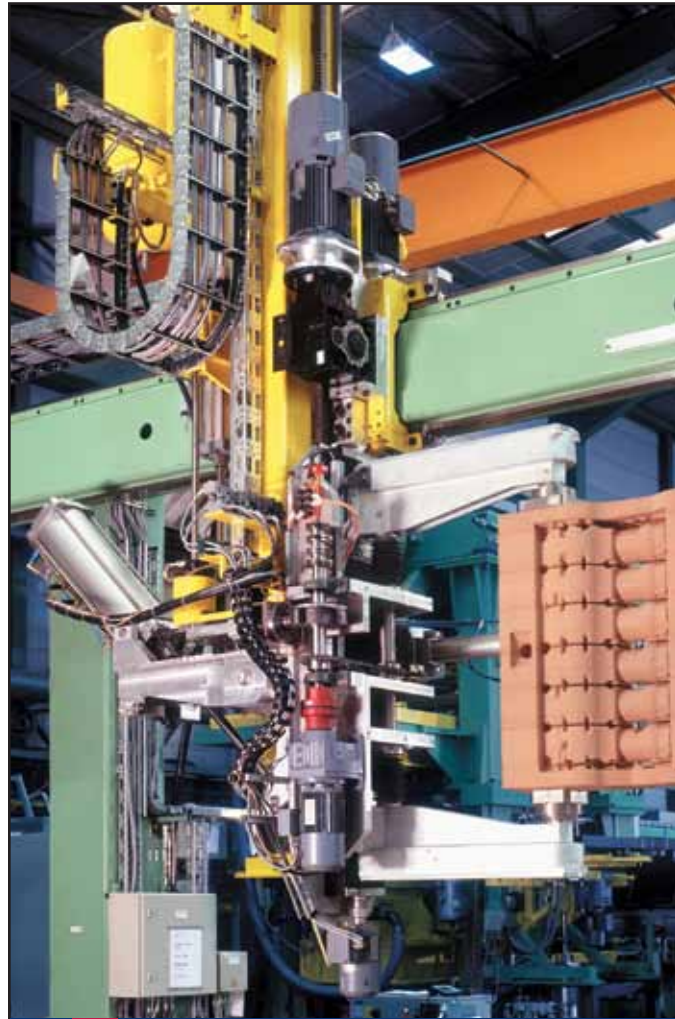
Product: VARITRAK S & ROBOTRAX Operating Mode: Vertical (loop-down) and 3D Application: Process Equipment
