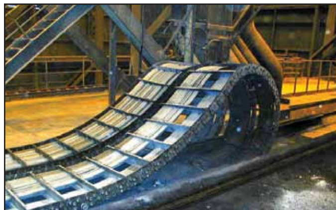
Product: VARITRAK S Operating Mode: Horizontal (RollerGlide KS , tandem) Application: Steel Mill Process Equipment
