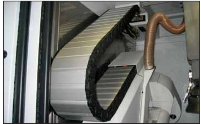
Product: VARITRAK MT with RMD aluminum lids Operating Mode: Horizontal (inclined) Application: Machining Center
