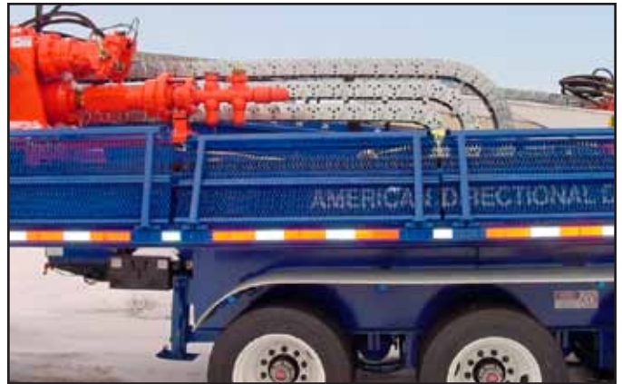
Product: VARITRAK S Operating Mode: Horizontal (triple nested with IDC KS ) Application: Horizontal Drilling and Boring 128
