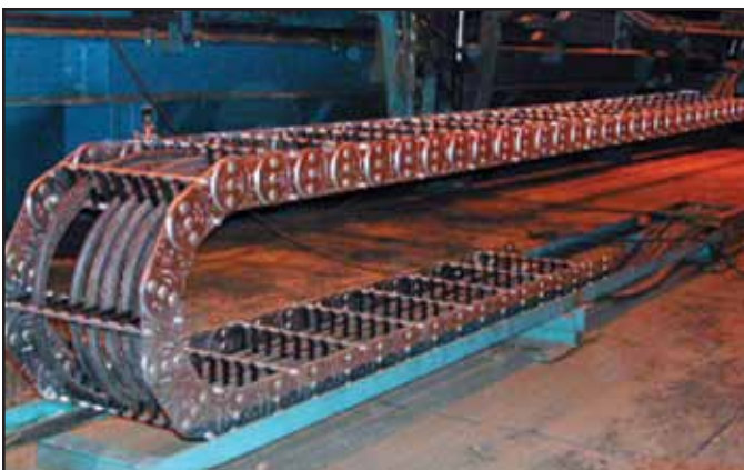
Product: VARITRAK S Operating Mode: Horizontal (on-the-floor) Application: Steel Processing Equipment
