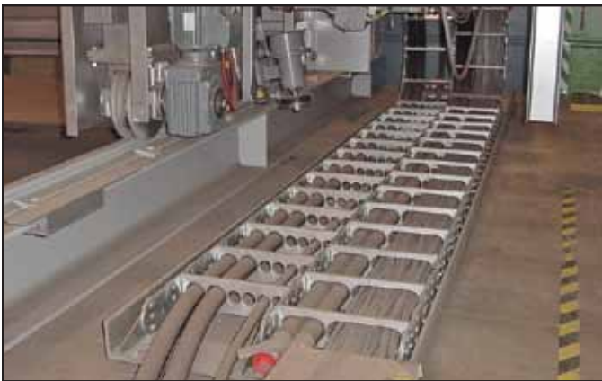
Product: VARITRAK S Operating Mode: Horizontal (on-the-floor, multi-chain-band) Application: Steel Mill Process Equipment
