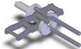
Open tail stock and adjust to the chain width
