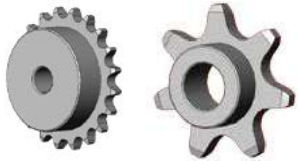
Figure 7 - Small and large roller double pitch sprockets
