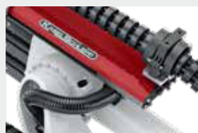
Active return mechanism with the PBU pull back unit (R040 - R100)
