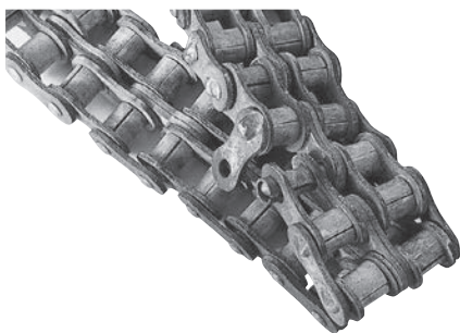
Corrosion of stainless steel drive chain
