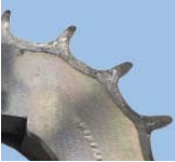
Standard stainless steel sprocket after use
