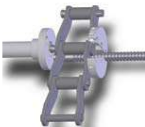
Ensure that there is enough room to adjust the chain pin position as needed
