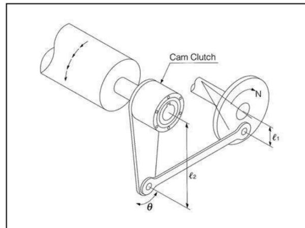
Figure 21: Critical dimensions for indexing applications
