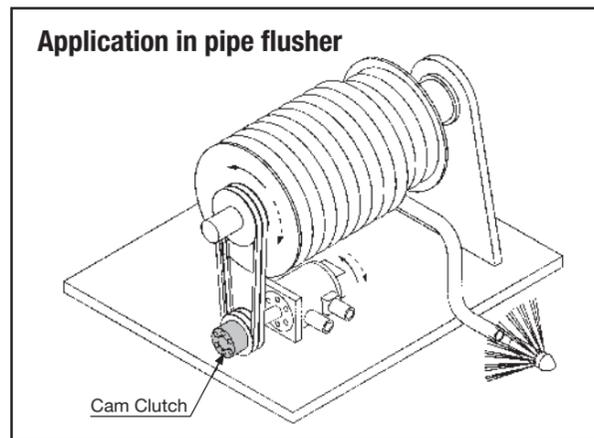
Figure 32: Pipe Flusher – Medium Overrunning Application
