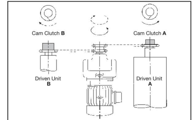
Figure 33: Selection based upon rotation direction
