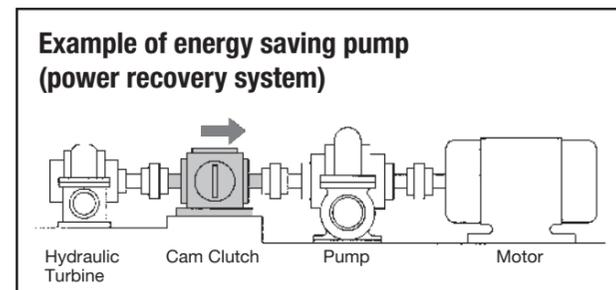
**Figure 24:** High-Speed Energy Saving Application
