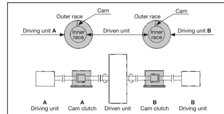
Figure 22: Dual Speed Drive System with Overrunning Cam Clutch
