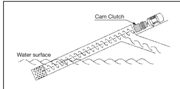
Figure 31: Inclined pump – Medium Overrunning Application
