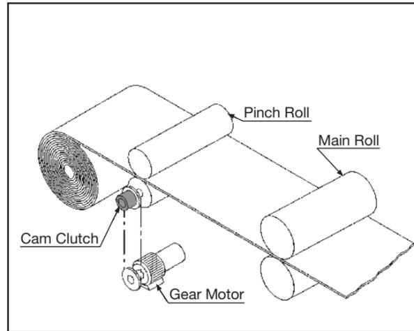
Figure 29: Feed roll – medium overrunning application
