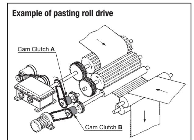
Figure 28: Two speed drive – Medium Overrunning and engagement
