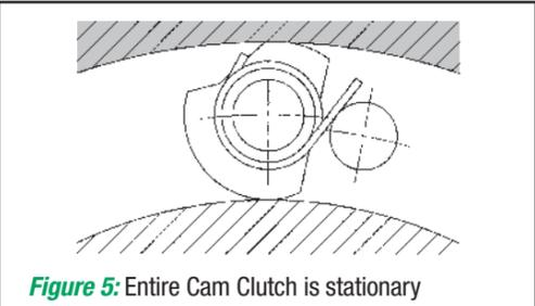
Figure 5: Entire Cam Clutch is stationary
