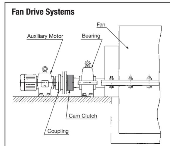
Figure 26: High-Speed/Low Engagement Energy Saving Application
