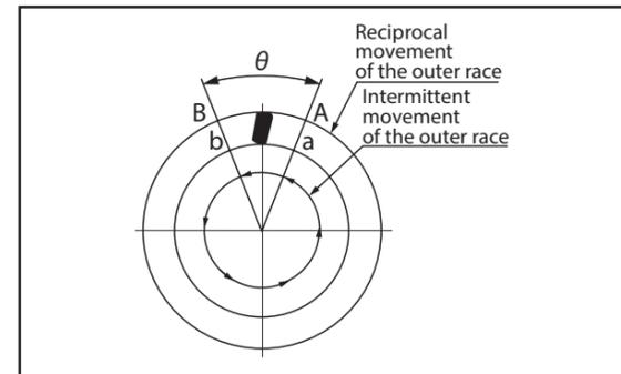
Figure 15: Cam Clutch inner and outer race interaction
