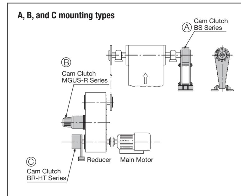
**Figure 9:** A,B,C backstop mounting
