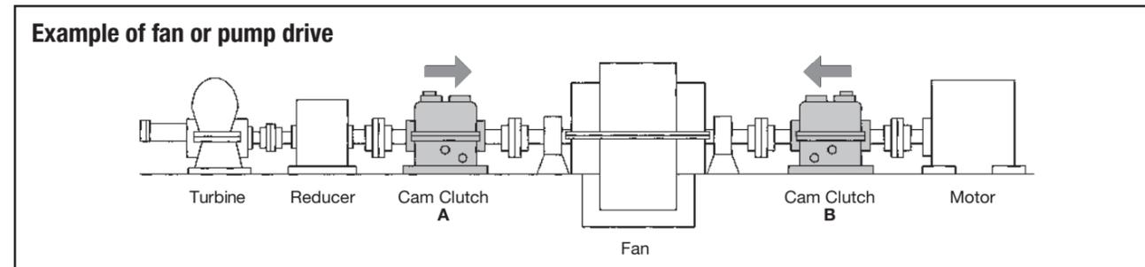
**Figure 23:** Typical High-Speed Overrunning Application
