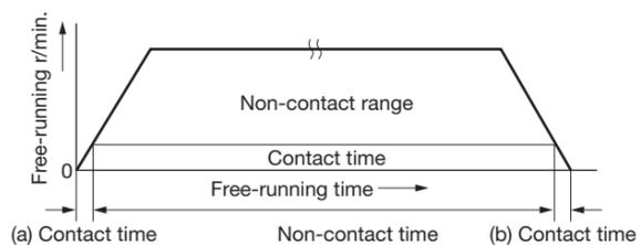
Friction in the clutch mechanism only occurs during a very short period of time denoted by "a" and "b". "a" is the time during which the cam is engaged until the acceleration of inner race causes it to disengage. "b" is the time during which the cam engages when the inner race decelerates.
