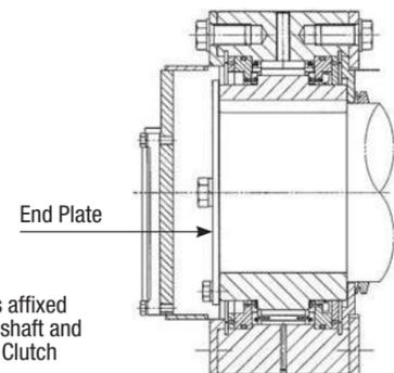
End plate is affixed to both the shaft and to the Cam Clutch
