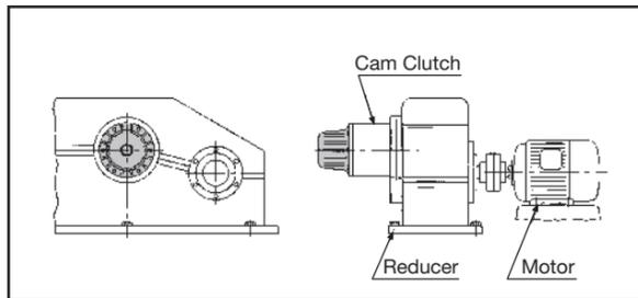
Figure 11: MGUS Series mounting medium speed
