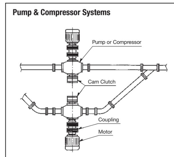
Figure 13: Cam Clutch installed on pump/compressor system
