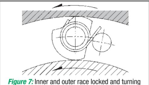
Figure 7: Inner and outer race locked and turning
