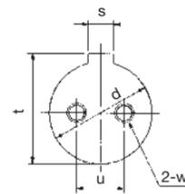
Dimensions detailing the end of the shaft are required so that Tsubaki can supply a matching plate
