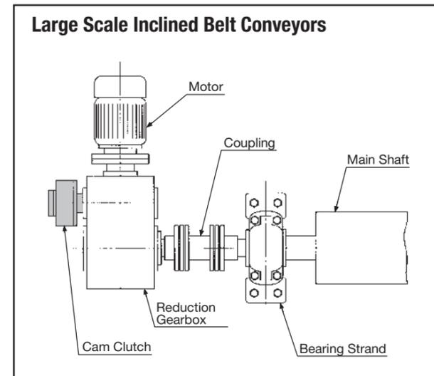
Figure 12: Cam Clutch installed on gear reducer
