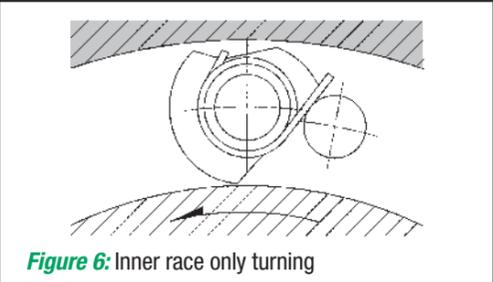
Figure 6: Inner race only turning
