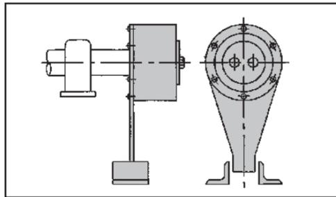
Figure 10: BS Series mounting low speed
