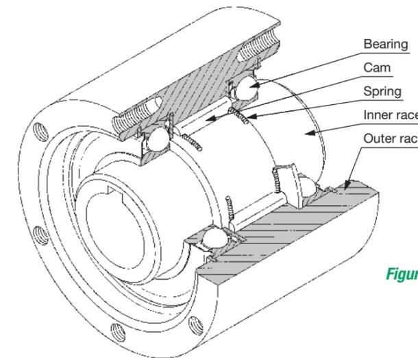
Figure 4: Cam Clutch major component parts
