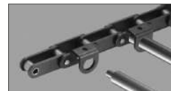
Stepped bar chain (Ends are inserted into holes in attachments)
