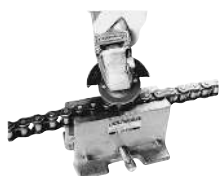
Figure 3: Grinding Down Pin Ends
