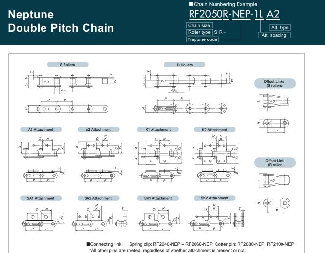
\*All other pins are riveted, regardless of whether attachment is present or not. \*Sizes over RF2080-NEP have cotter pins on both ends of the offset link.
