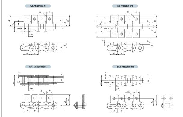
Connecting link: Spring clip: RS40-NEP – RS60-NEP Cotter pin: RS80-NEP – RS100NEP \*All other pins are riveted, regardless of whether attachment is present or not.
