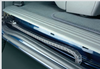
Rocker solution: Wire track under running board in vertical or horizontal position.
