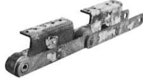
3. Wear from Corrosion
