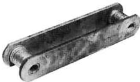
2. Wear from Conveyed Materials
