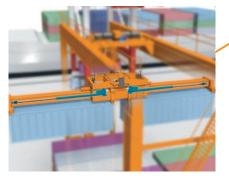
Arm Extension Adjusts the length of the arm to match the size of the container (such as for double containers).
