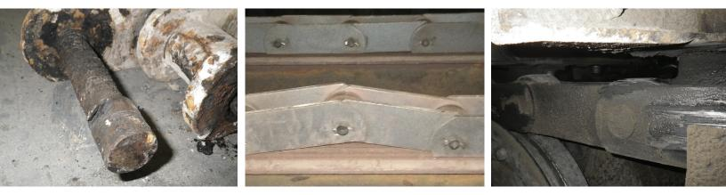
Tsubaki's patented SJ3 Sealed Joint Technology effectively protects and defends a chain's bearing areas by impeding the infiltration of aggressive fine and sticky particulate. In doing so, the risks of premature elongation, joint lockage and/or dry cavitation are greatly reduced, thus allowing for more effective chain performance and extended life.
