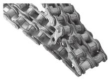
Corrosion of stainless steel drive chain
